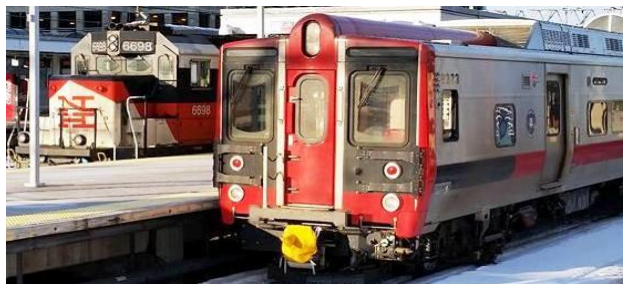
Diesel-hauled SLE service at New Haven. Right: M8 EMU that will replace the diesel-hauled equipment.
